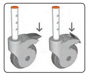
To lock the castor wheels press down firmly on the end of brake with your foot. This will lock the castor so that it will not move or rotate.
