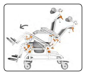
While squeezing the brake handle the chair can be returned to the upright position.
