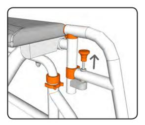
To swing-away or remove the footrest pull up on the knob which will unlock the footrest position.
