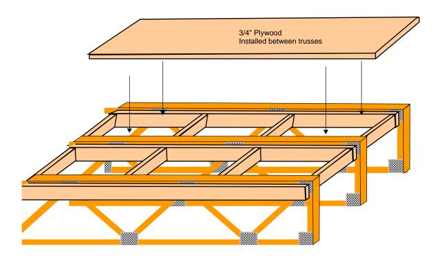
Install 2x4's to the side of engineered trusses, 3/4" down from the top of the truss. Provide 2x4 cross bracing on each end and every 16"-24". Cross bracing should also be provided under the existing sub-floor to eliminate deflection. Cut 3/4" plywood to fit between trusses and secure in place.
